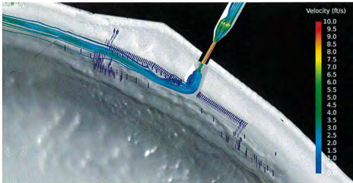
Figure 18 – Streamlines colored by velocity with Alternative 1 docking facility and operating diversion.
